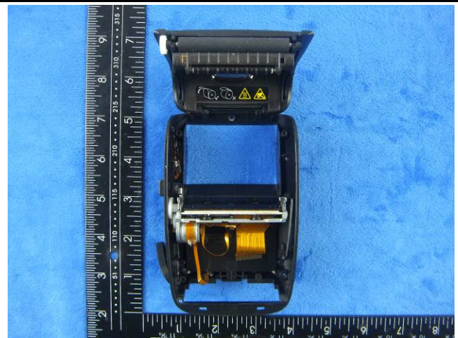
Motor - Front View
