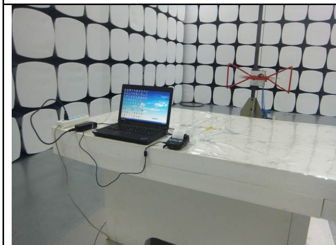
Conducted Emissions Test Setup – Front View
