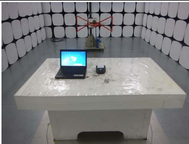
Radiated Spurious Emissions Test Setup Below 1GHz
