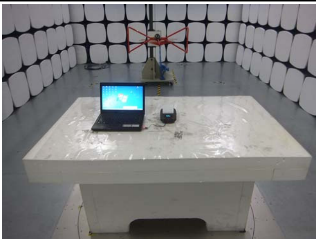
Radiated Spurious Emissions Test Setup Below 1GHz
