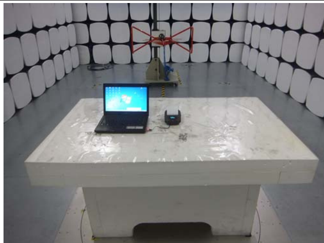
Radiated Spurious Emissions Test Setup Below 1GHz
