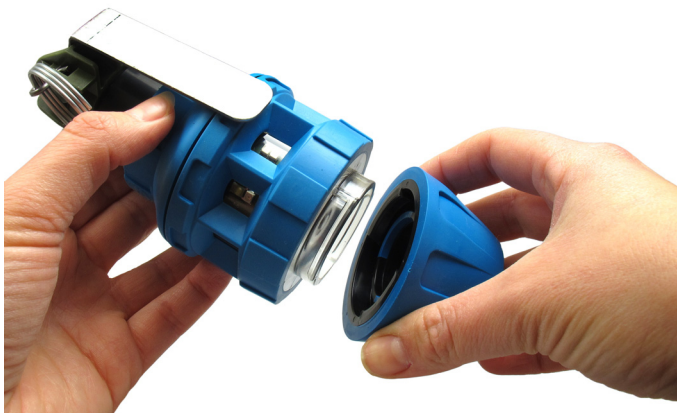
Fig 13. Pyro unit removal
