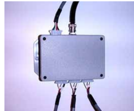
Figure 13 - Antenna Cable to Matching Board Box Connection
