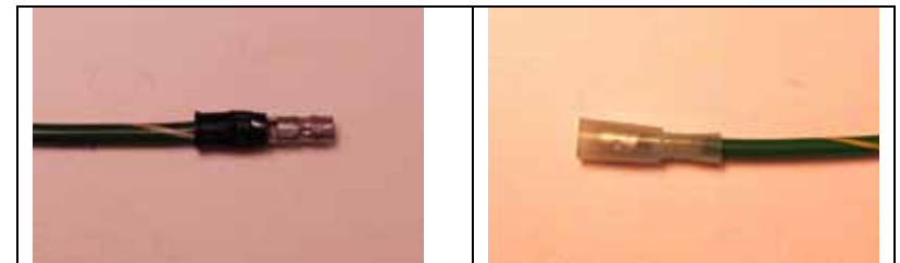
Figure 23 - Grounding Wire Connectors
