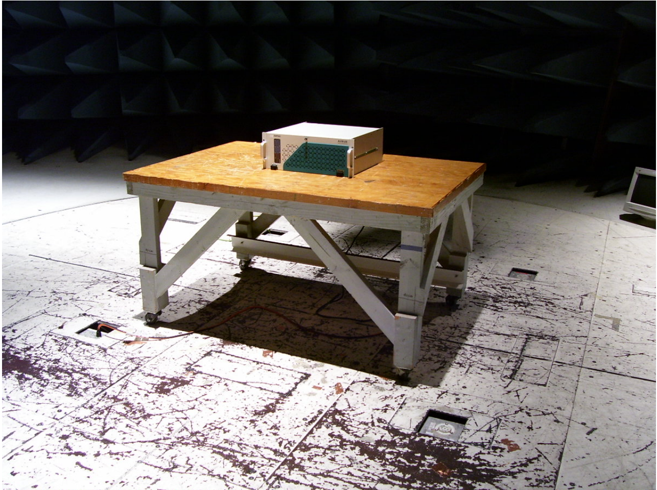
Photograph 3. Radiated Emission Limits Test Setup
