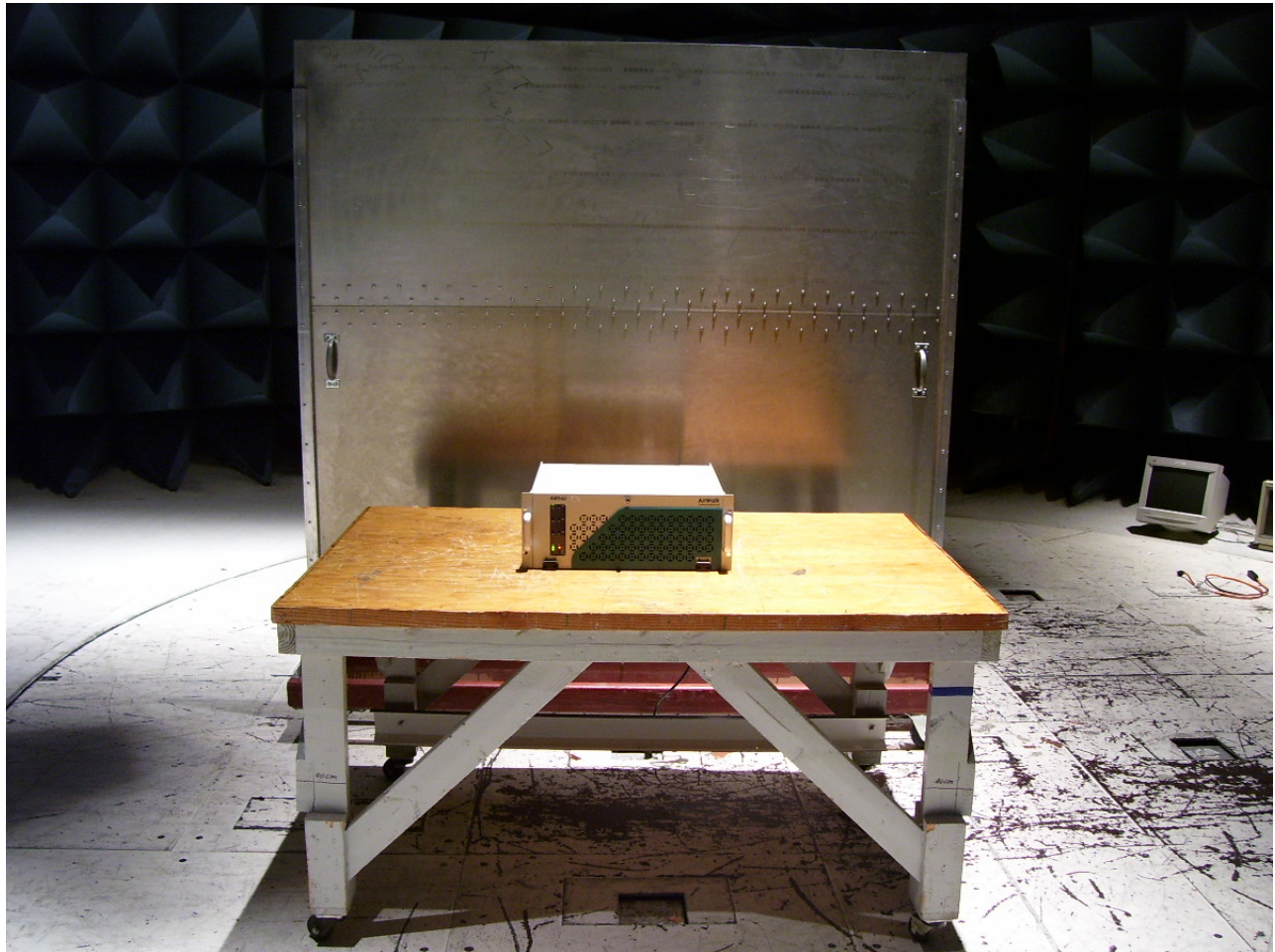
Photograph 2. Conducted Emissions Test Setup
