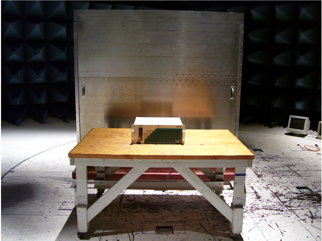
Photograph 2. Conducted Emissions Test Setup
