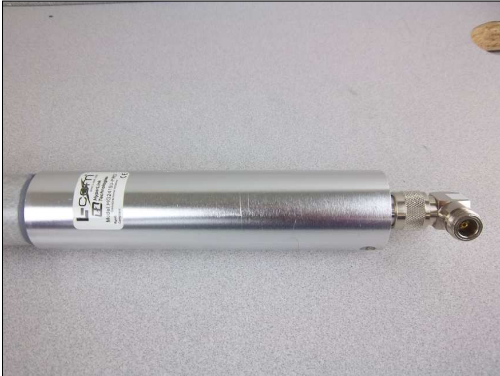
Figure 8: External Photo – Omni-Directional Antenna
