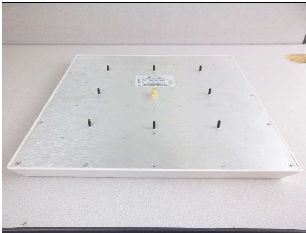
Figure 6: External Photo – Panel Antenna
