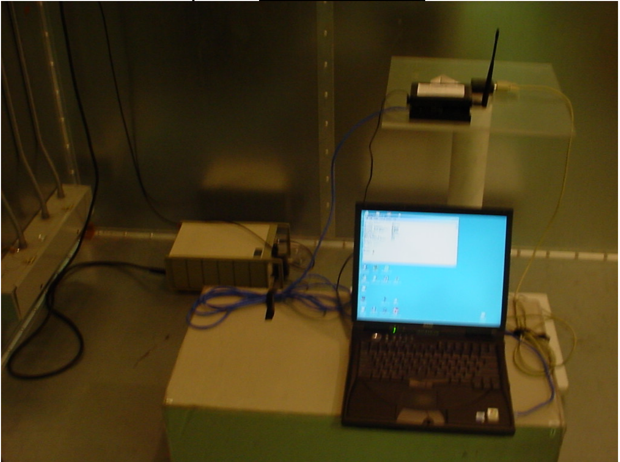
Setup for the Conducted Emissions Test
