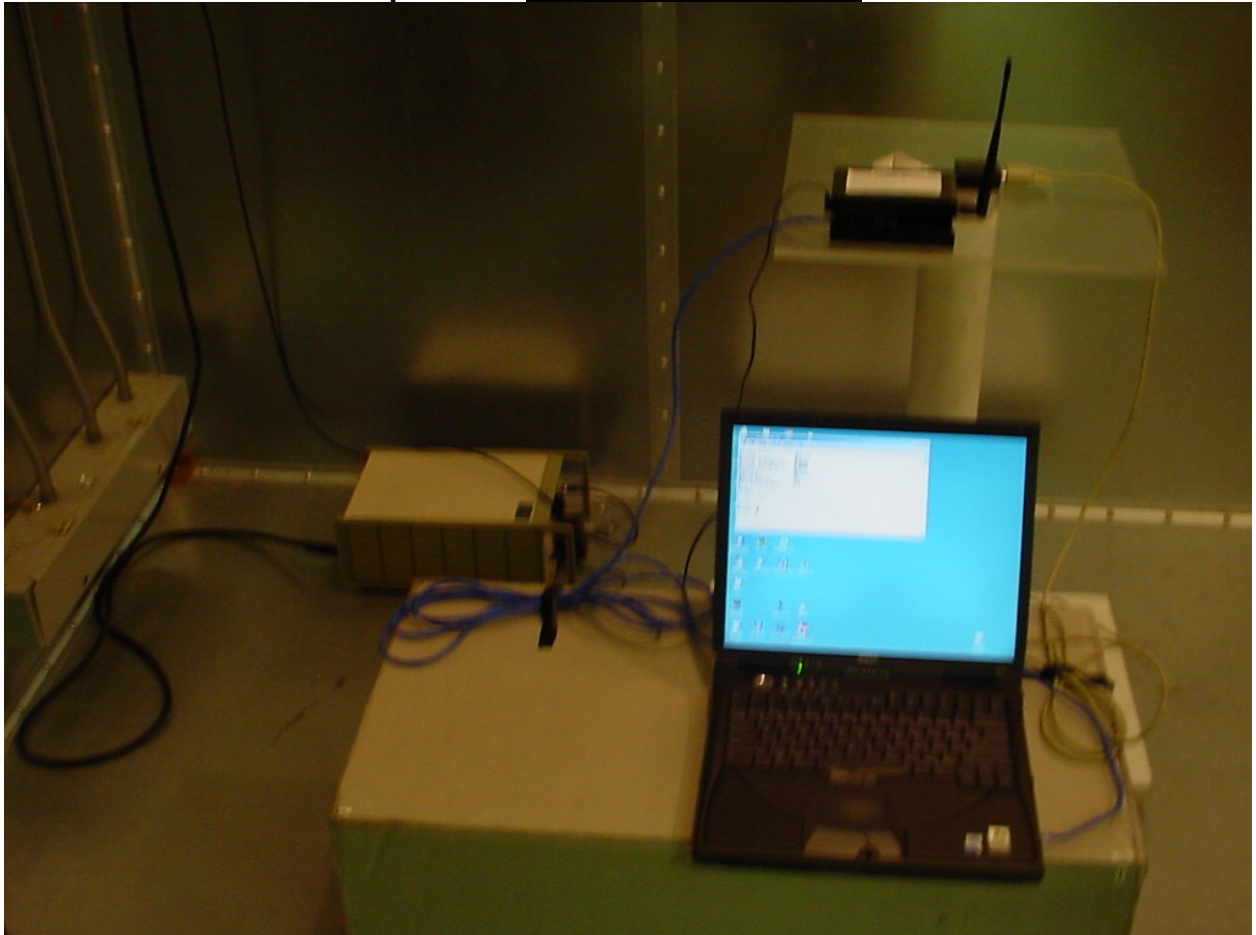
Setup for the Conducted Emissions Test
