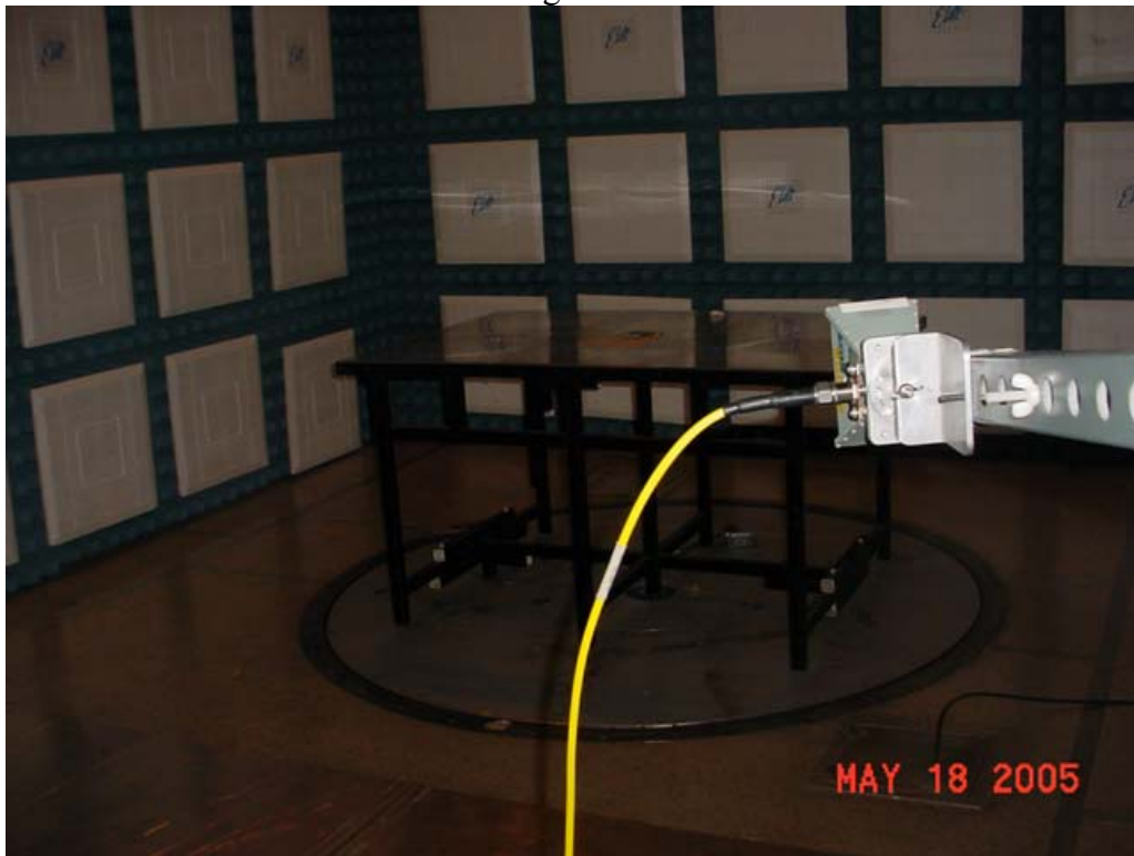
Test Set-up for Radiated Emissions – Horizontal Polarization
