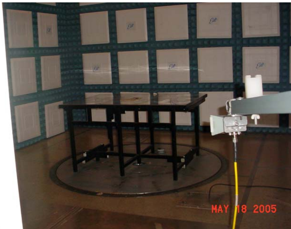
Test Set-up for Radiated Emissions – Vertical Polarization
