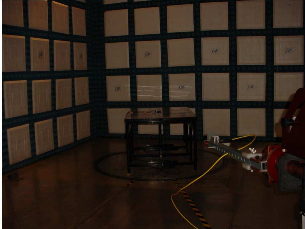
Test Set-up for Radiated Emissions – Horizontal Polarization
