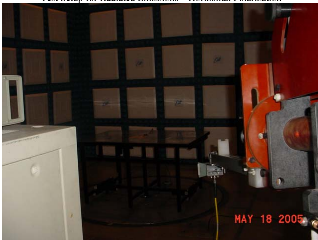
Test Setup for Radiated Emissions – Vertical Polarization
