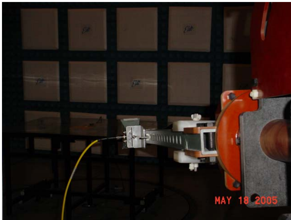
Test Setup for Radiated Emissions – Horizontal Polarization
