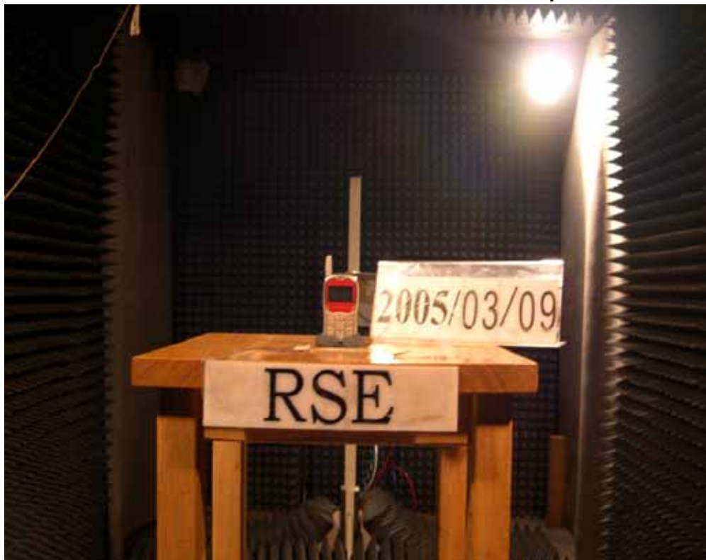
TCL538 Radiated Spurious Emission Test Setup
