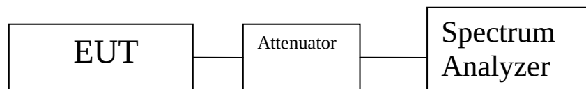
Figure 3. Block Diagram, Conducted Spurious Emissions Test Setup
