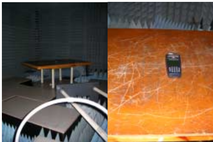
Photograph 7.2.1 Setup for spurious emission field strength measurements below 30 MHz
