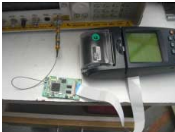
Photograph 7.1.1 Peak output power test setup
