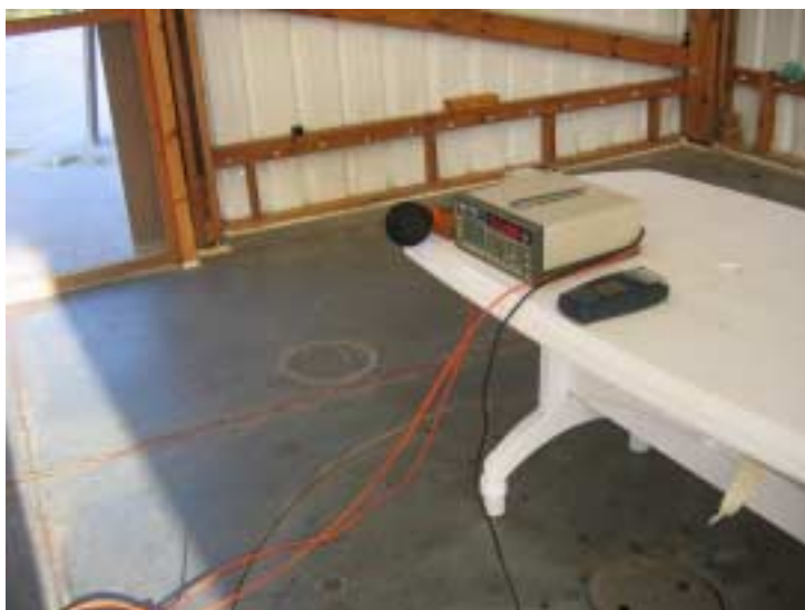
Photograph 7.3.1 Maximum permissible exposure (MPE) measurement set up
