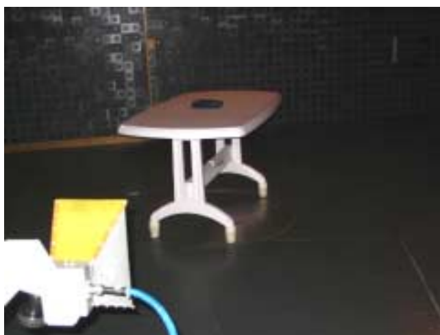
Photograph 7.2.4 Setup for spurious emission field strength measurements, close view
