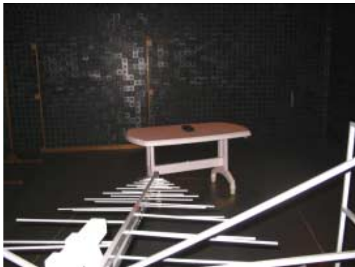
Photograph 8.1.1 Setup for radiated emission measurements
