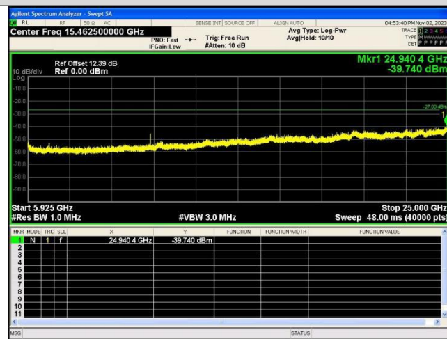
Spurious Emission:5925~25000.0 MHz IEEE 802.11a_Channel 149_20MHz_Antenna 0
