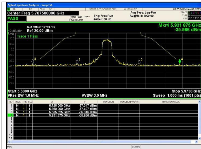
Out Of Band Emission IEEE 802.11n_Channel 157_20MHz_Antenna 0
