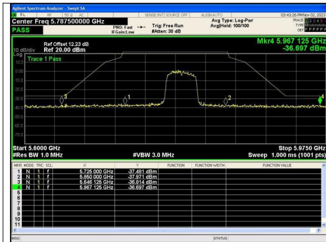
Out Of Band Emission IEEE 802.11ac_Channel 159_40MHz_Antenna 0
