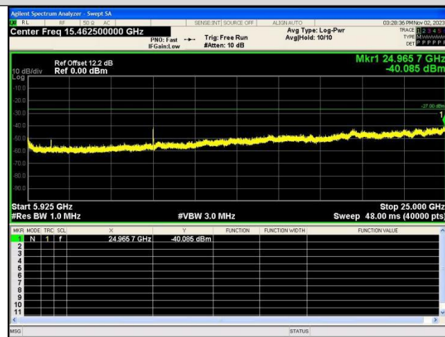
Spurious Emission:5925~25000.0 MHz IEEE 802.11ac_Channel 165_20MHz_Antenna 0
