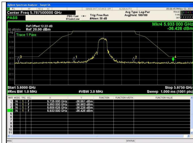
Out Of Band Emission IEEE 802.11n_Channel 157_20MHz_Antenna 0
