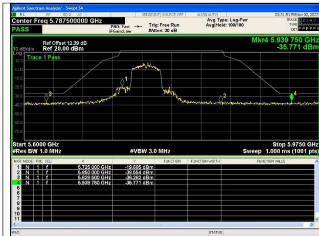
Out Of Band Emission IEEE 802.11n_Channel 151_40MHz_Antenna 0
