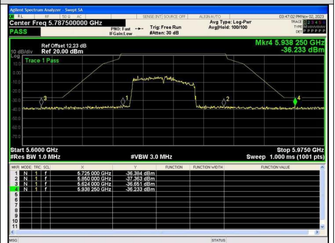
Out Of Band Emission IEEE 802.11ac_Channel 155_80MHz_Antenna 0
