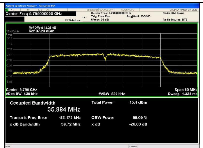
IEEE 802.11n_Channel 159_40MHz_Antenna 0
