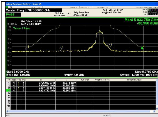
Out Of Band Emission IEEE 802.11a_Channel 165_20MHz_Antenna 0
