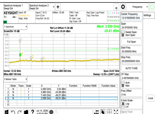
Spurious Emission \pi/4 DQPSK 2M DH5 2480MHz
