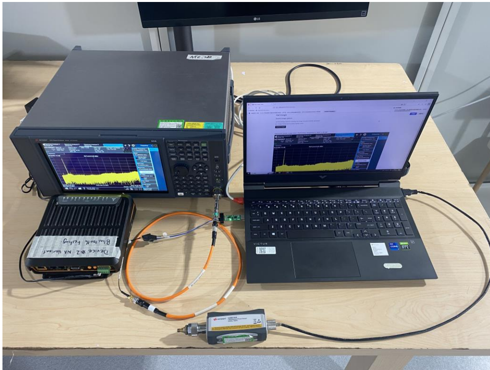
Description: DFS Test Setup
