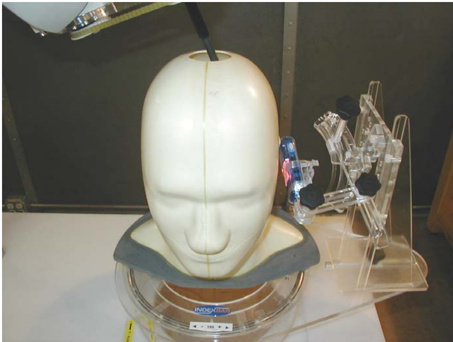
Figure S1. Setup Configuration of Left Ear Cheek and Tilt ( 850/1900 Head SAR)
