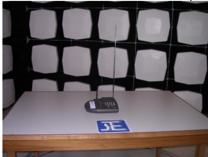
Measurement of Conducted Emission Test Set Up
