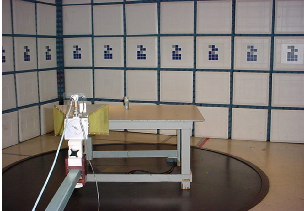
Radiated Test Set-up Front View (1)
