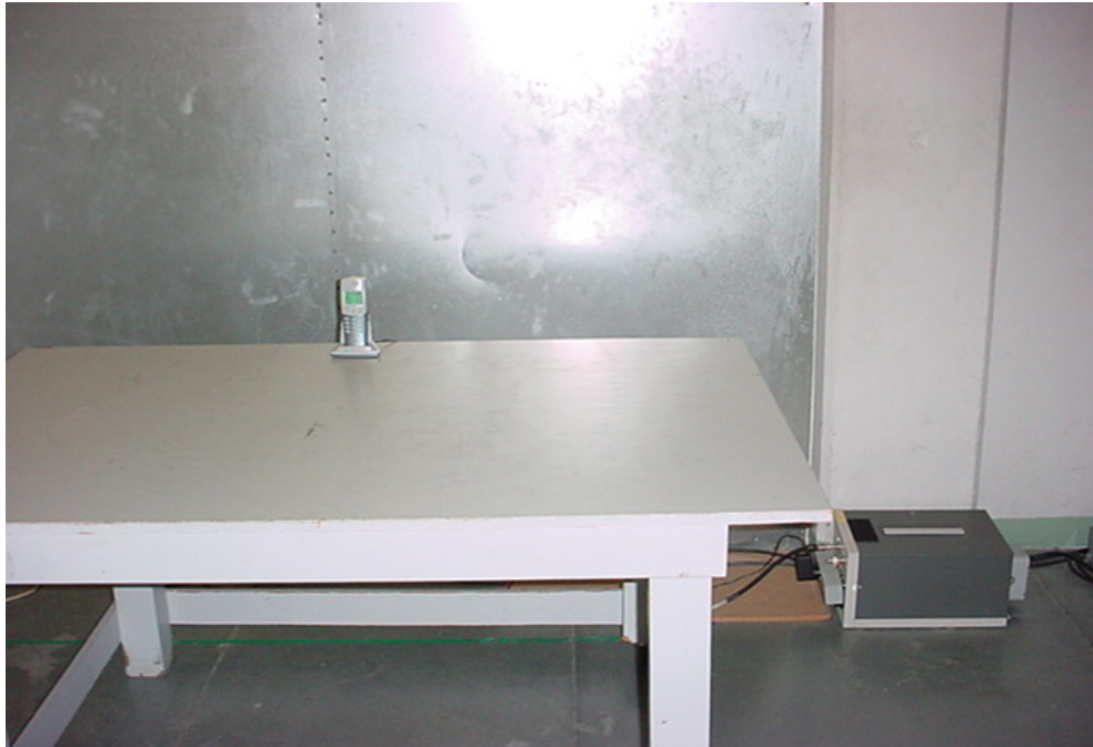
AC Line Conducted Emission Test Set-up Front View
