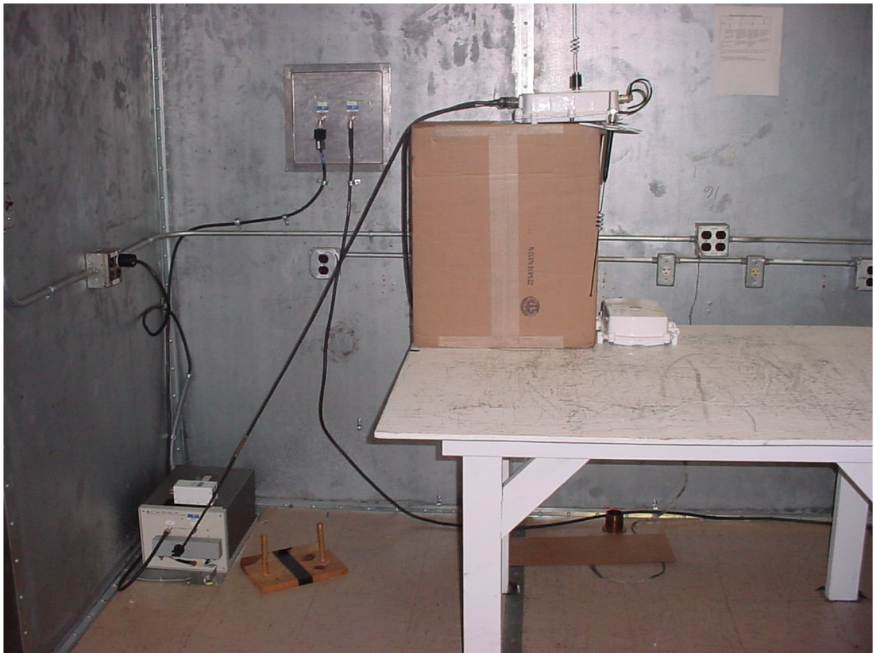
Figure 5: Test Setup – Conducted Emissions
