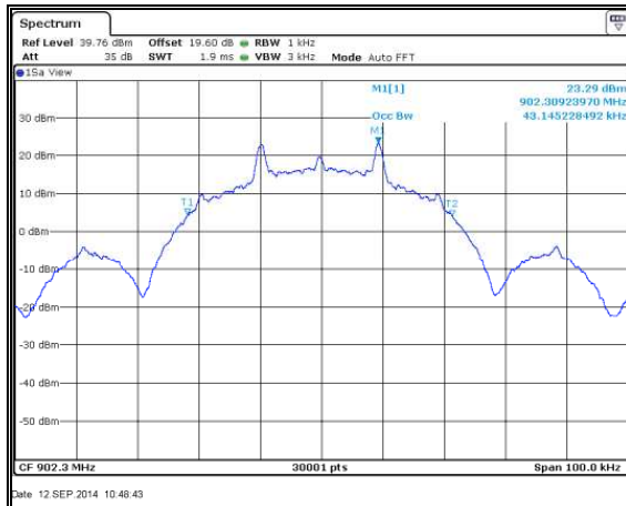
Figure 7.4.4.2-23: 99% BW Low Channel - 19.2kbps
