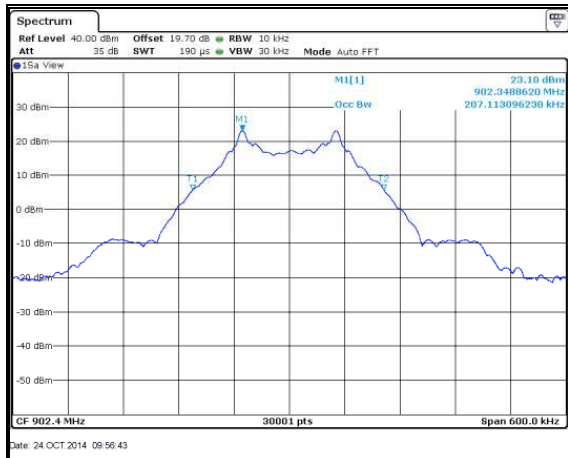
Figure 7.4.4.2-28: 99% BW Low Channel – 200.0kbps
