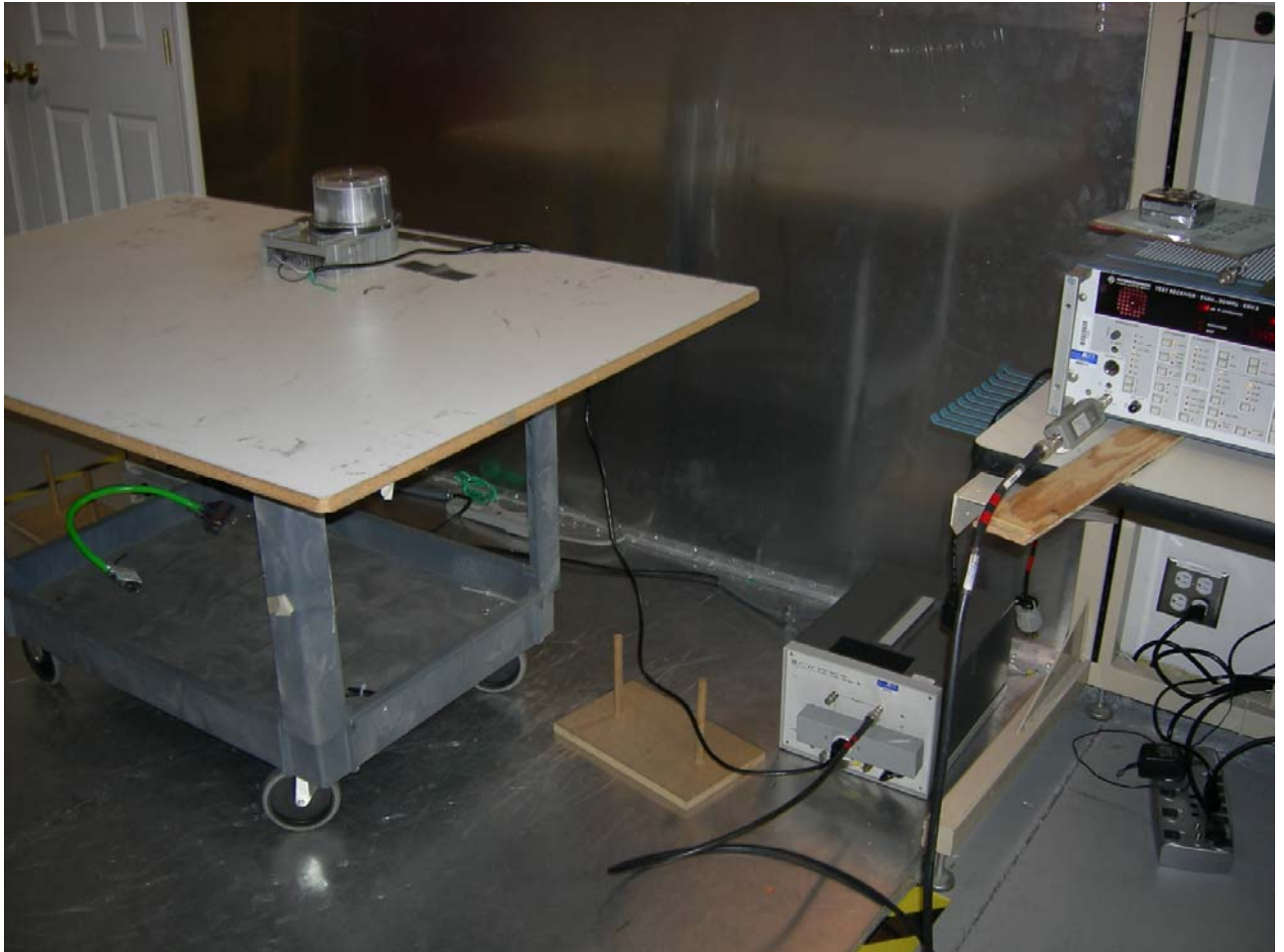
Figure 5: Test Setup - Conducted Emissions
