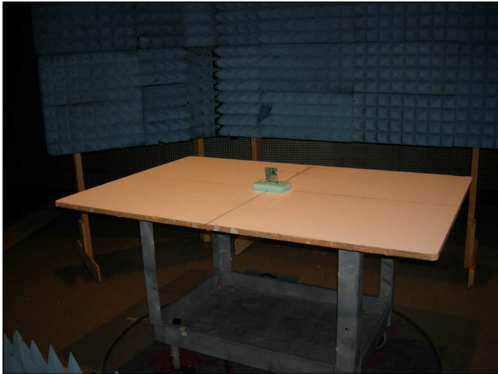
Figure 1: Test Setup Photo - Radiated Emissions
