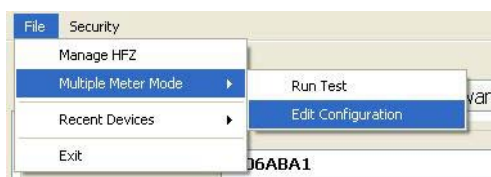
Figure 3 - 25. Accessing Multiple Meter Test Configuration
