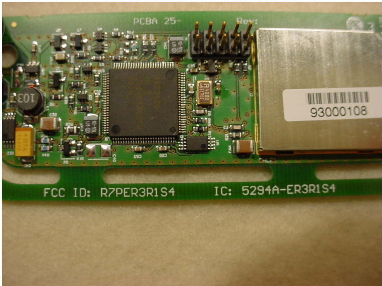
Figure 1: Label Information: Module Label and Location
