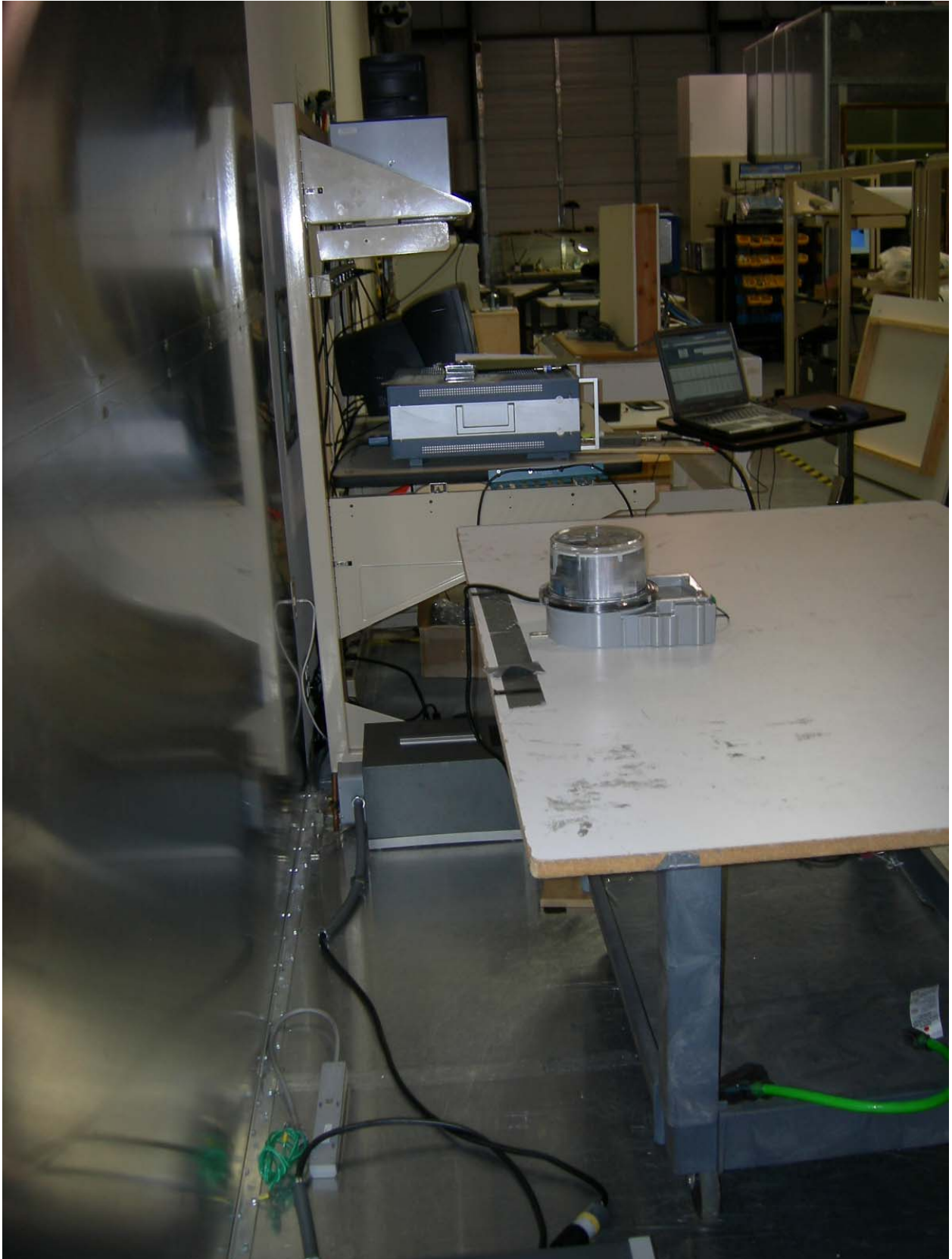
Figure 6: Test Setup - Conducted Emissions
