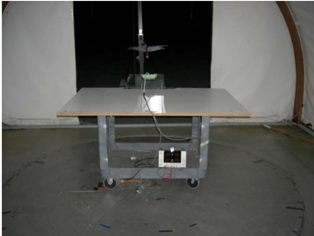
Figure 3: Test Setup - Radiated Emissions – Unintentional
