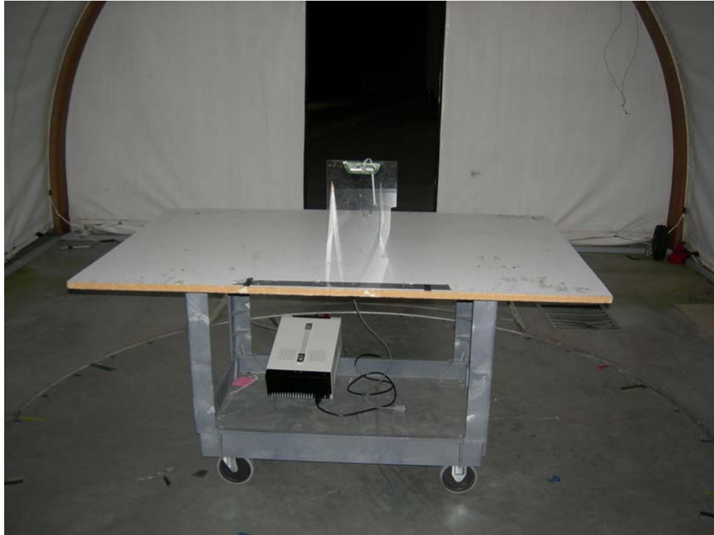
Figure 4: Test Setup - Radiated Emissions – Unintentional
