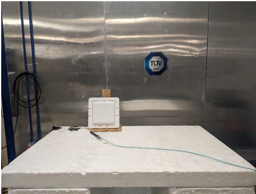
Figure 14 – Test Set up – Conducted Emissions – Sector Antenna
