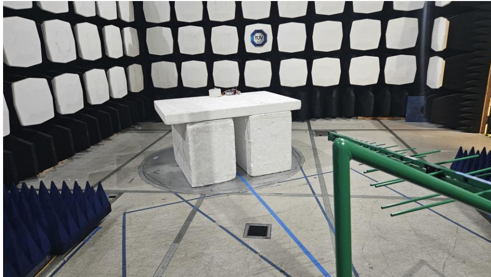
Figure:3 – Test Set up – Front View of the EUT- Radiated Emissions <1 GHz
