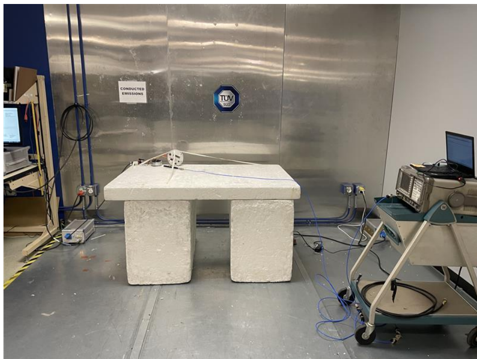
Figure:12– Test Set up – Front View of the EUT - Conducted Emissions
