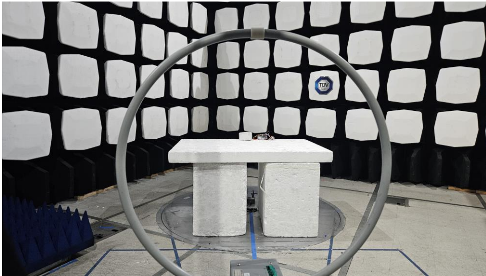
Figure:1 – Test Set up – Front View of the EUT - Radiated Emissions <30 MHz
