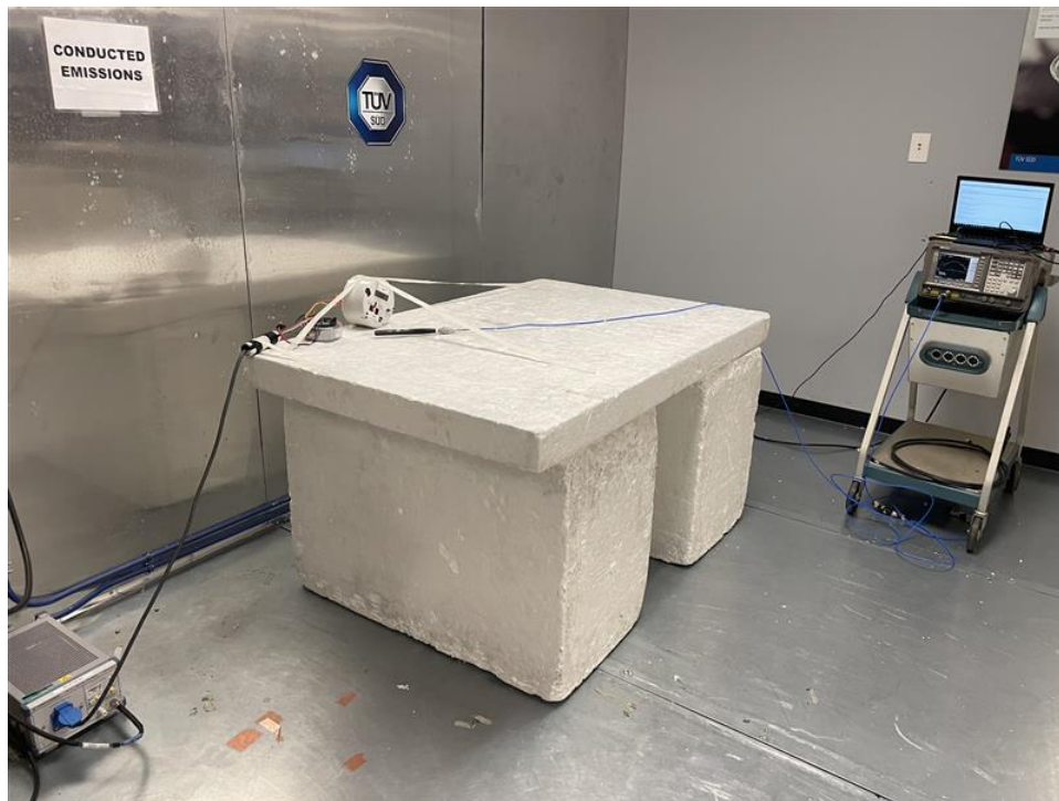
Figure:11– Test Set up – Side View of the EUT - Conducted Emissions
