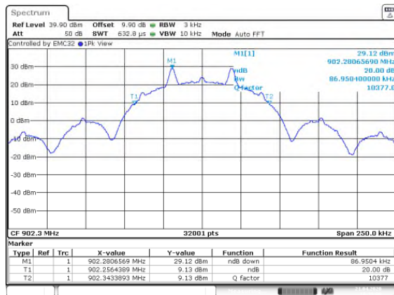
Figure 7.4.4.2-3: 20dB BW Low Channel - 38.4kbps
