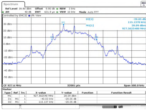
Figure 7.4.4.2-20: 20dB BW High Channel – 150.0kbps
