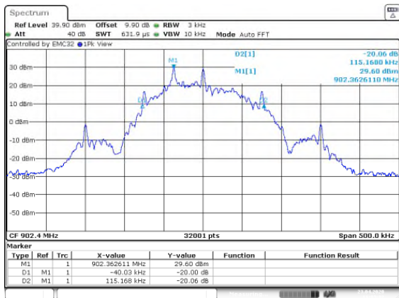
Figure 7.4.4.2-6: 20dB BW Low Channel - 150.0kbps
