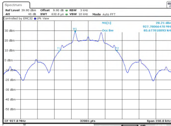
Figure 7.4.4.2-38: 99% BW High Channel – 38.4kbps
