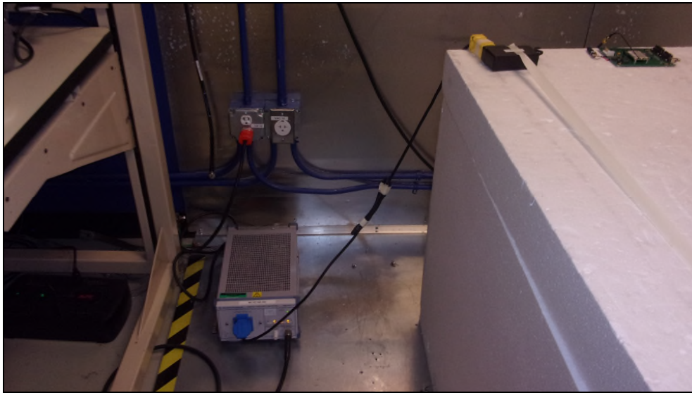
Figure 11: Equipment Under Test – AC Conducted Emissions
