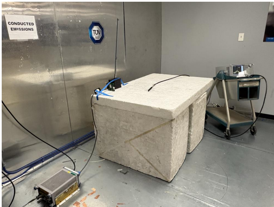
Figure:7– Test Set up – Side View of the EUT - Conducted Emissions
