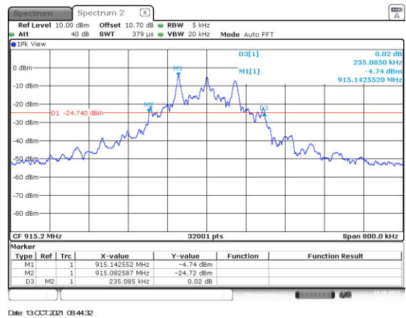
Figure 2.3.6-8: 20dB BW Mid Channel – 115.2 kbps
