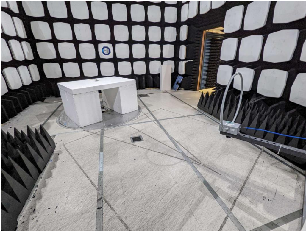
Figure 2: Equipment Under Test – Radiated Emissions <30MHz
