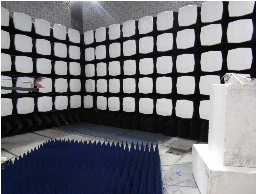
Figure:3 – Test Set up - Radiated Emissions <10 GHz
