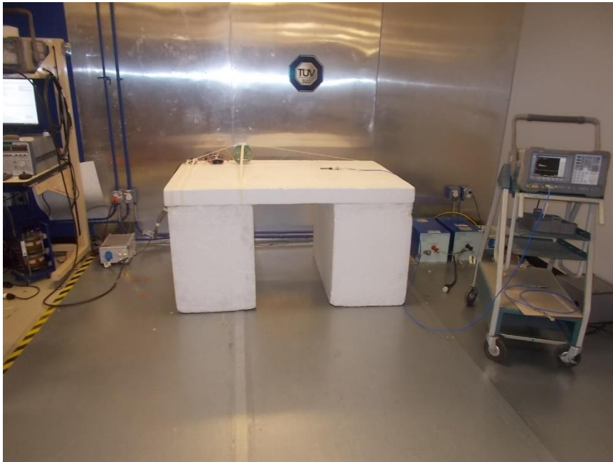
Figure:5 – Test Set up – Conducted Emissions
