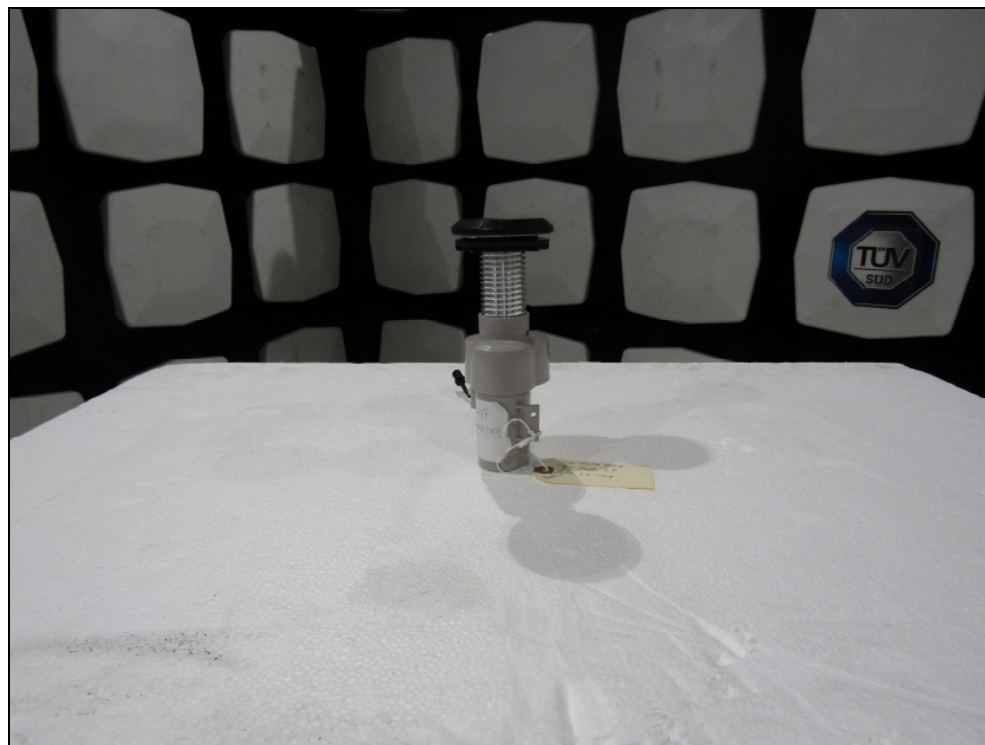
Figure 2: Equipment Under Test – Radiated Emissions Metal Antenna Sleeve
