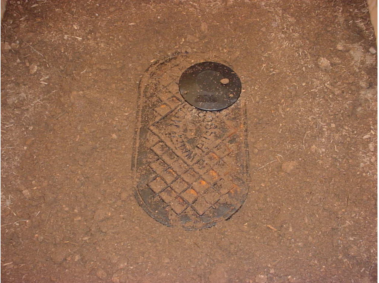
Figure 3: Test Setup – Radiated Emissions (Intentional – Cast Iron Meter Box)
