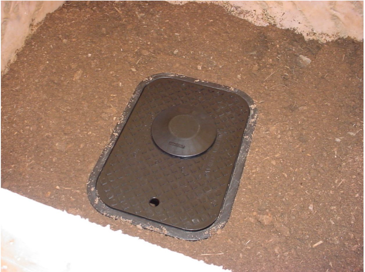
Figure 1: Test Setup – Radiated Emissions (Intentional – Composite Meter Box)
