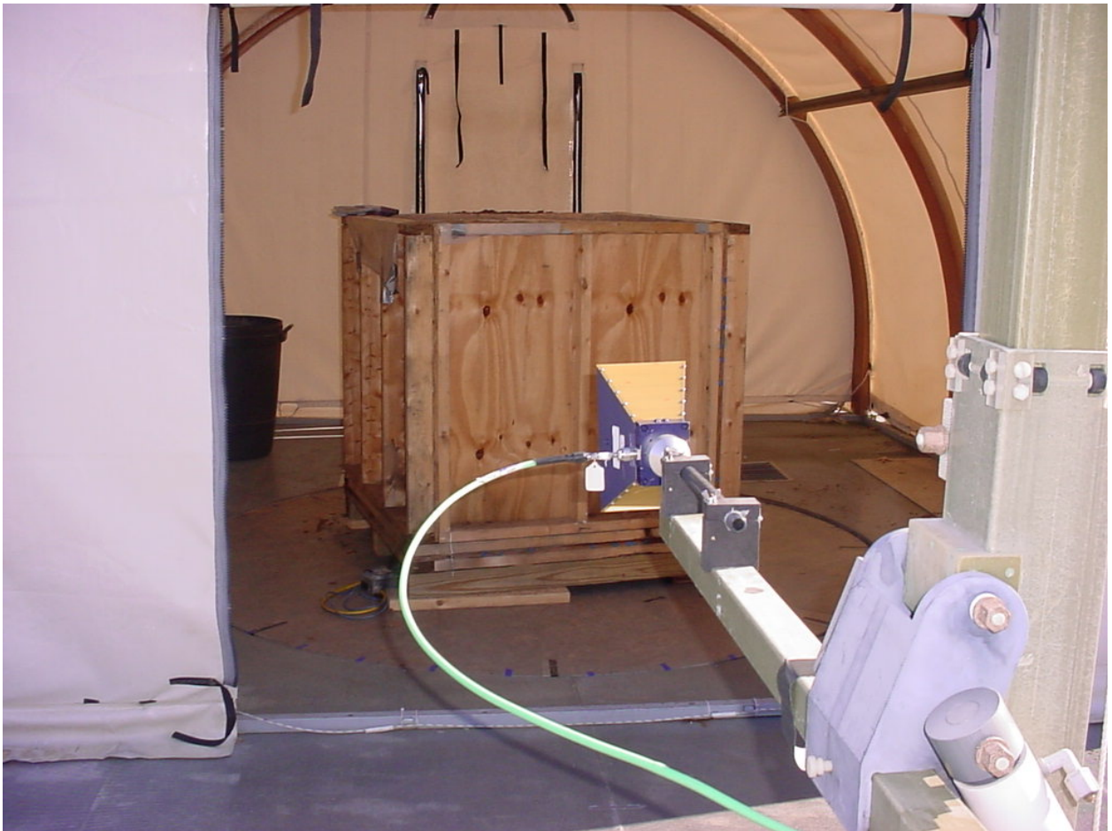
Figure 1: Test Setup – Radiated Emissions (Intentional – Wood Test Fixture Exterior)
