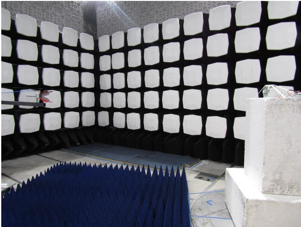
Figure3 – Test Set up - Radiated Emissions <10 GHz
