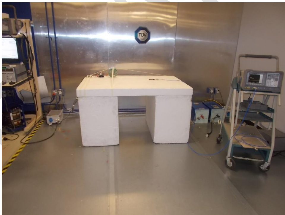
Figure6 – Test Set up – Conducted Emissions
