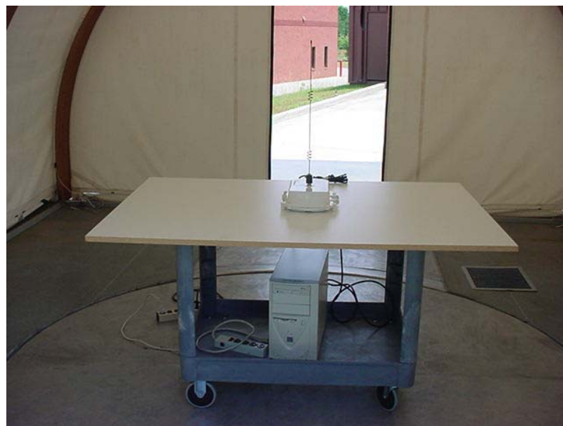
Figure 2: Radiated Emissions – WANGATE with UTILINET DC RADIO Front View
