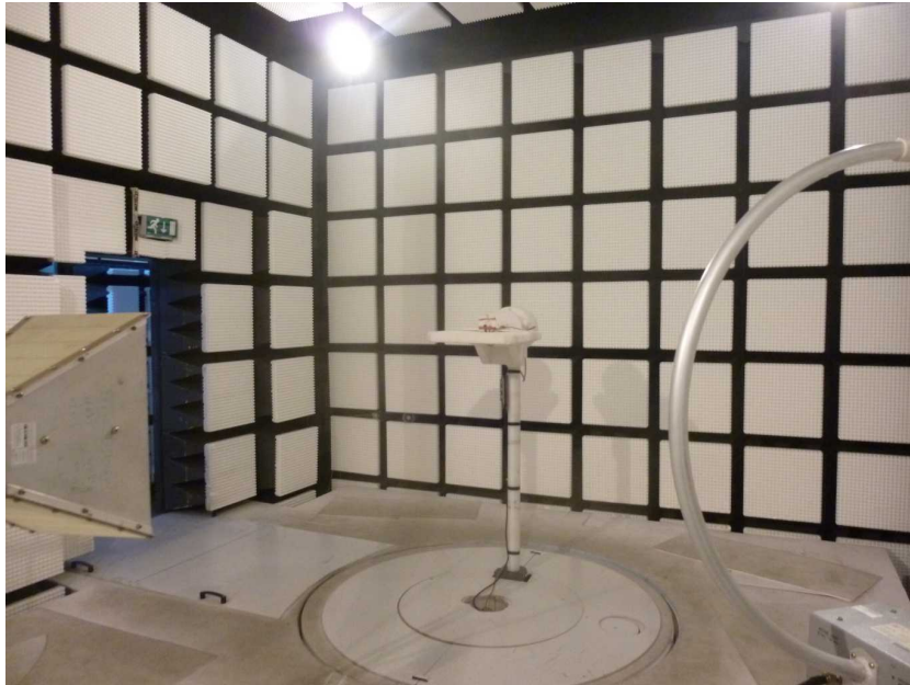
Photo 7: EUT at the anechoic chamber, stand-alone module with integrated antenna
