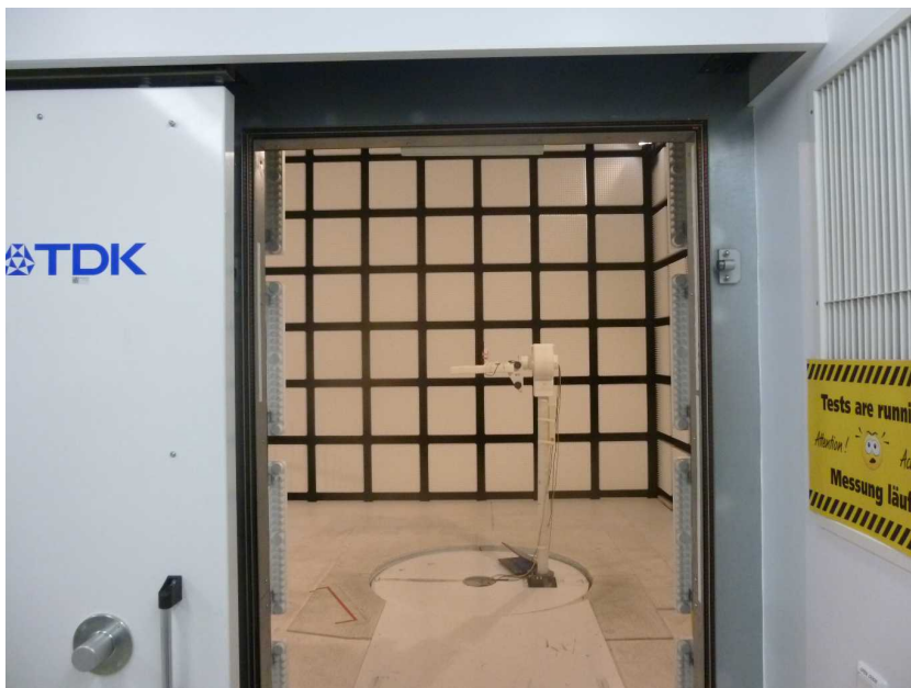
Photo 8: EUT at the anechoic chamber, module with external antenna
