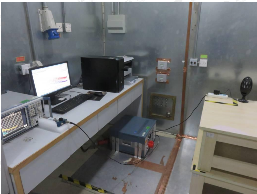
FCC RADIATED EMISSION TEST SETUP
