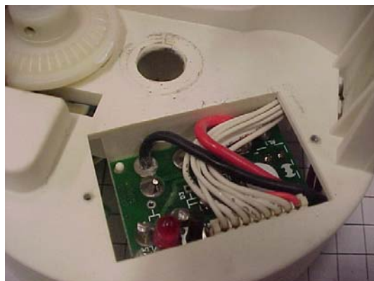
PHOTO N° 4 – INTERNAL VIEW: RECEIVER MODULE AND ANTENNA
