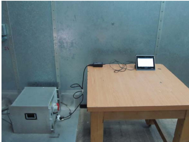
Photo 7. Conducted emissions test setup.
