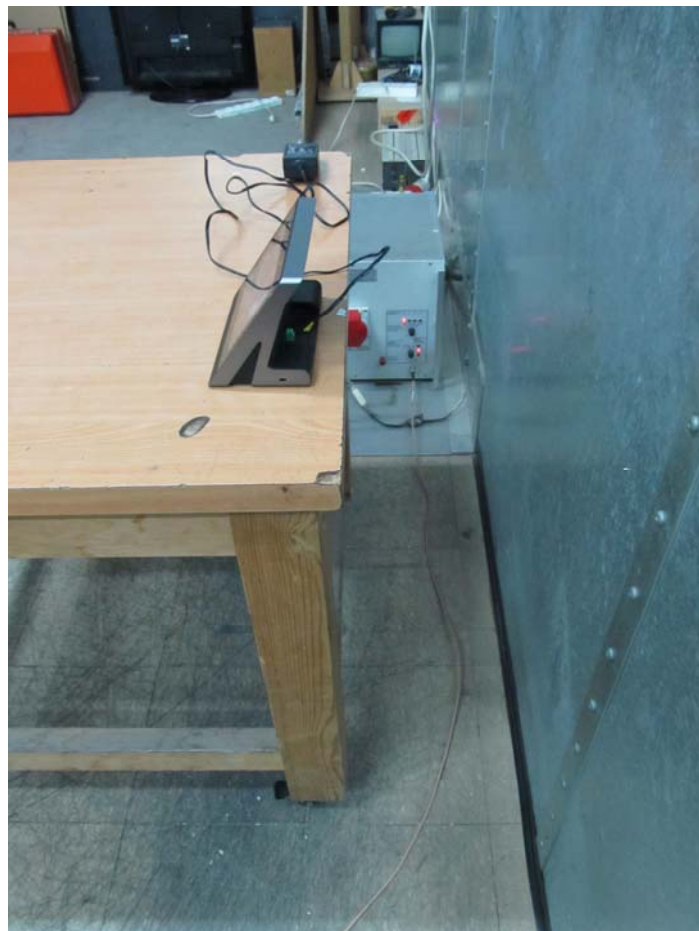
Photo 8. Conducted emissions test setup.
