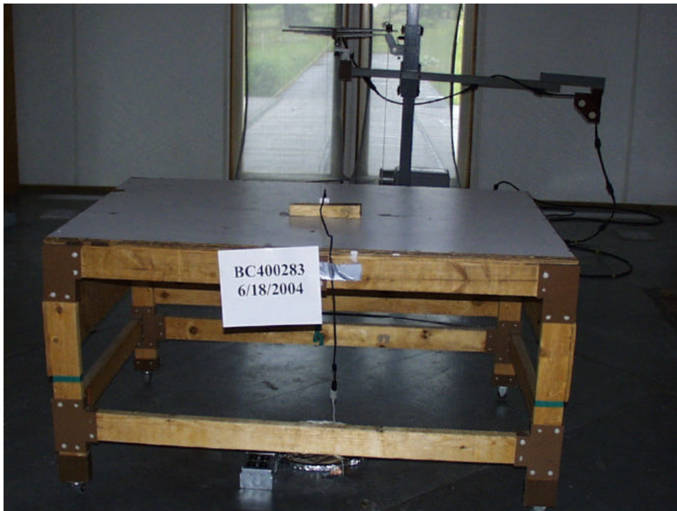
Test-setup photo(s): Radiated Emissions
