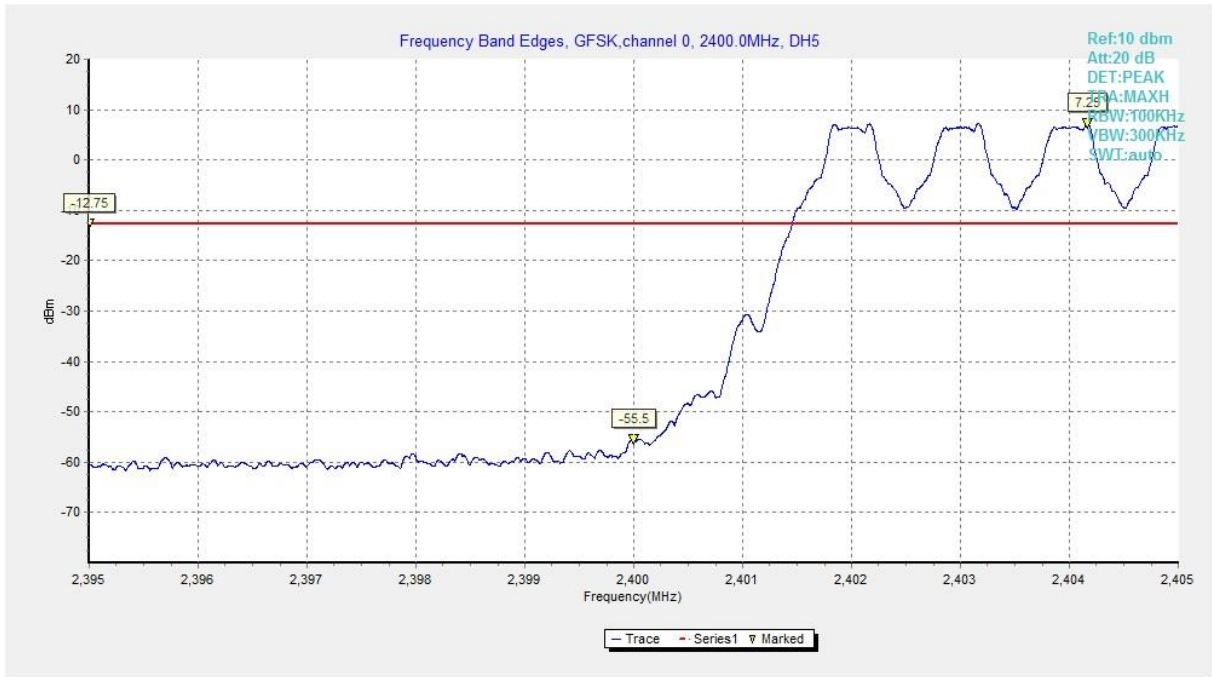
Fig. 1 Band Edges (GFSK, CH0, Hopping ON)
