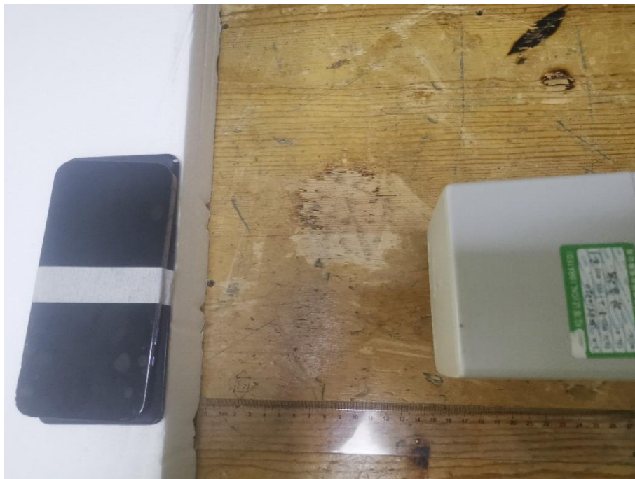
E-Field&amp;H Filed Test Setup Photo of Position Right (15cm)
