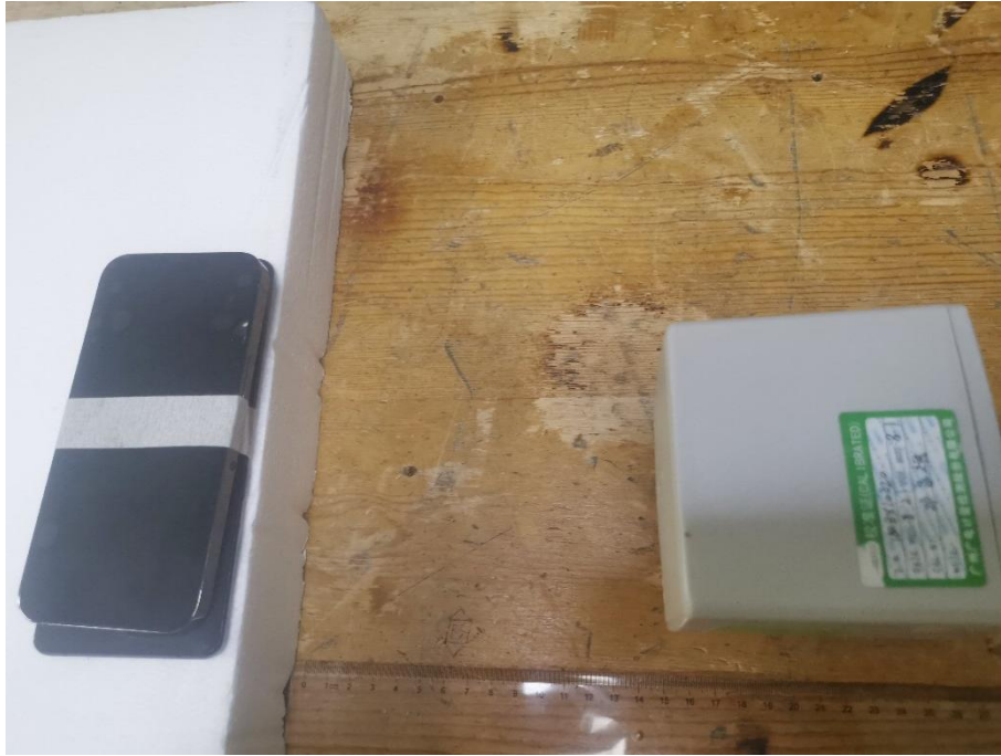
E-Field&amp;H Filed Test Setup Photo of Position Left (15cm)
