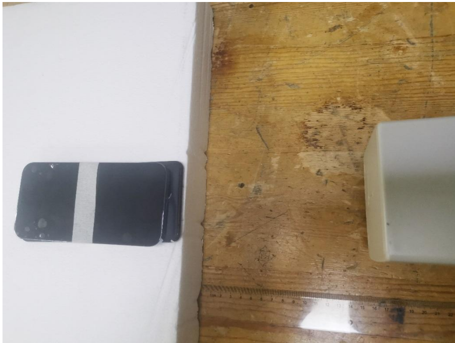
E-Field&H Filed Test Setup Photo of Position Front (15cm)
