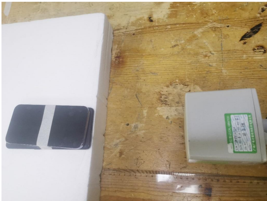
E-Field&H Filed Test Setup Photo of Position Back (15cm)
